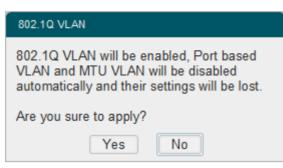
3) In the **802.1Q VLAN Setting** section, enter a VLAN ID and a VLAN name for identification to create a VLAN. Select the untagged port(s) and the tagged port(s) respectively to add to the created VLAN based on the network topology. Click **Apply**.
