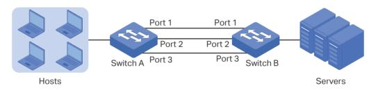
Demonstrated with TL-SG1016PE, the following section provides configuration steps. The configuration steps are similar for both switches, here we take Switch A for example.
