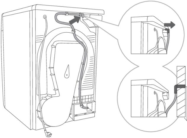
**1** Release the hose from the holder on the back wall of the dryer (left hand side, below the top cover).
