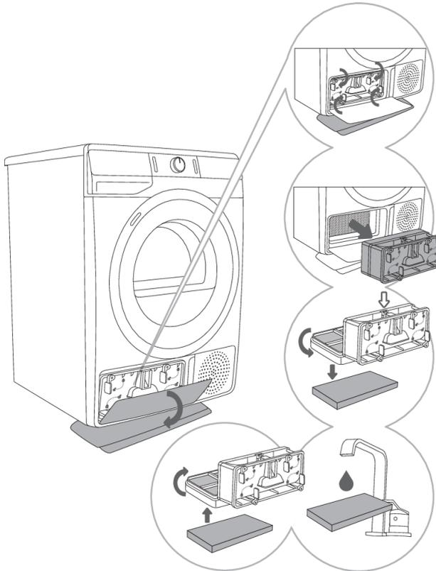
**1** Open the outside cover. Hold the levers on the inside cover and rotate them as indicated by the arrows.
